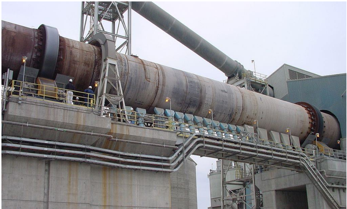
Figure 5.1 Line diagram of rotary kiln for the manufacture of cement
