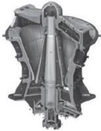
Figure 8.3 Cut section of Fuller-Traylor gyratory crusher. (Courtesy FLSmidth Minerals).
