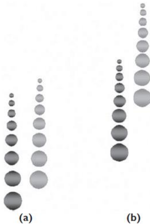
Figure 12.1 (a) Free settling; (b) Hindered settling.
