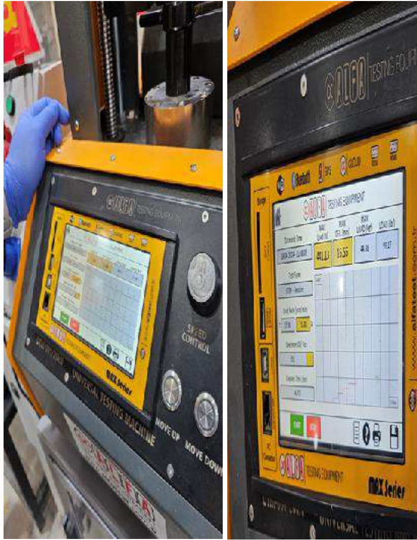
Figure9: Photographic image shows Alfa Universal Testing Machine (Model UTM-001 Turkey) with 20kN capacity.
