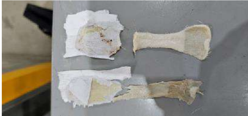
Figure10: Photographic image shows the tearing of both acellular tissue sampler after completing the mechanical testing.
