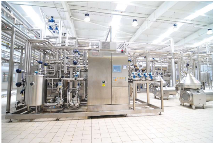
Basic Flow - HTST Pasteurization
