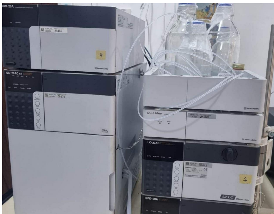
Figure 12: device of HPLC(High-performance liquid chromatography )
