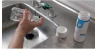
Photo 2. Rinsing with de-ionized water
