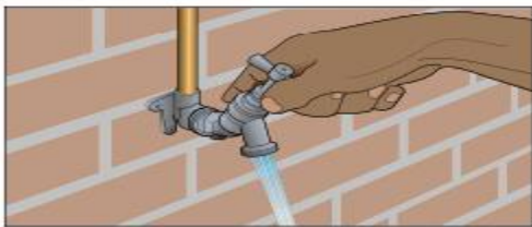
Figure 5. Open the tap until it reaches its maximum rate of flow
