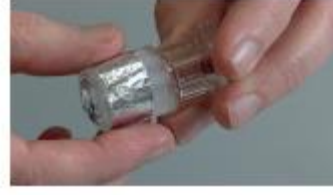
Photo 4. A strip of aluminium foil to prevent the stopper from sticking during sterilization
