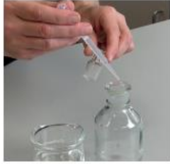
Photo 3. Adding a few drops of aqueous sodium thiosulphate solution
