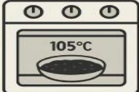
Place it in an oven at 105°C for 24 hours, or in the sun until fully dry.
