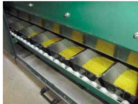
Bucket elevator with pastilles.
