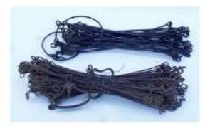
The chain survey is the simplest method of surveying. In the chain survey, only measurements are taken in the field, and the rest work, such as plotting calculation, etc. are done in the office. Here only linear measurements are made i.e. no angular measurements are made. This is most suitably adapted to small plane areas with very few details. If carefully done, it gives quite accurate results.
