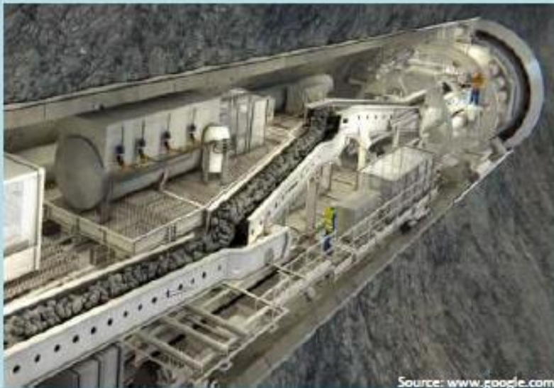
(c) Conveyor belt Excavation
