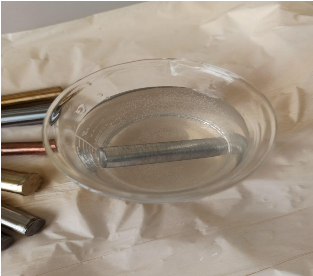
Fig. (2-5) Shows uncoated Specimens into Sulfuric Acid.
