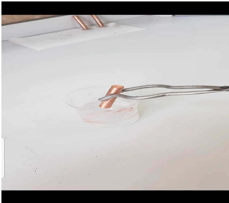
Fig. (2-1): coating of selected metals by (Epoxy).
