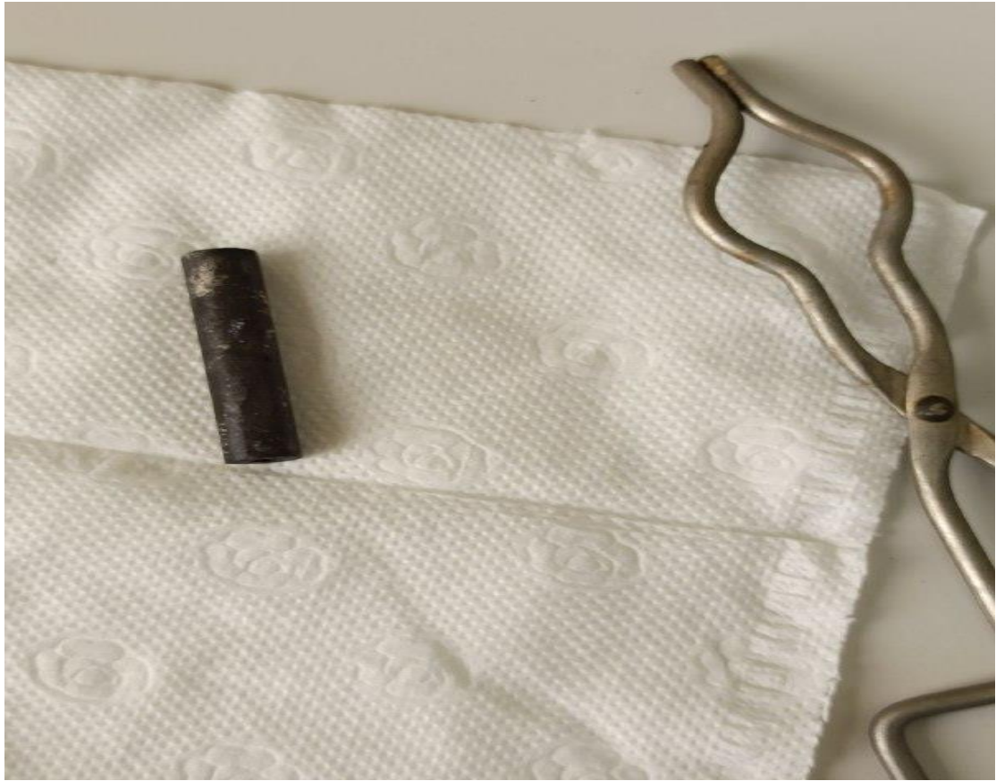
Fig. (2-9) Shows the Corrosion of The Specimens.
