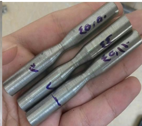
Fig. (8) Shows Geometry of specimen of carbon steel
