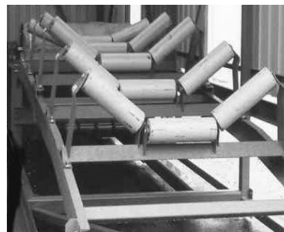
Fig. 6.1.7. Three roll idler : Sketch shows three roll carrying idler with straight return idler in same frame, and photograph shows set of assembled idlers
