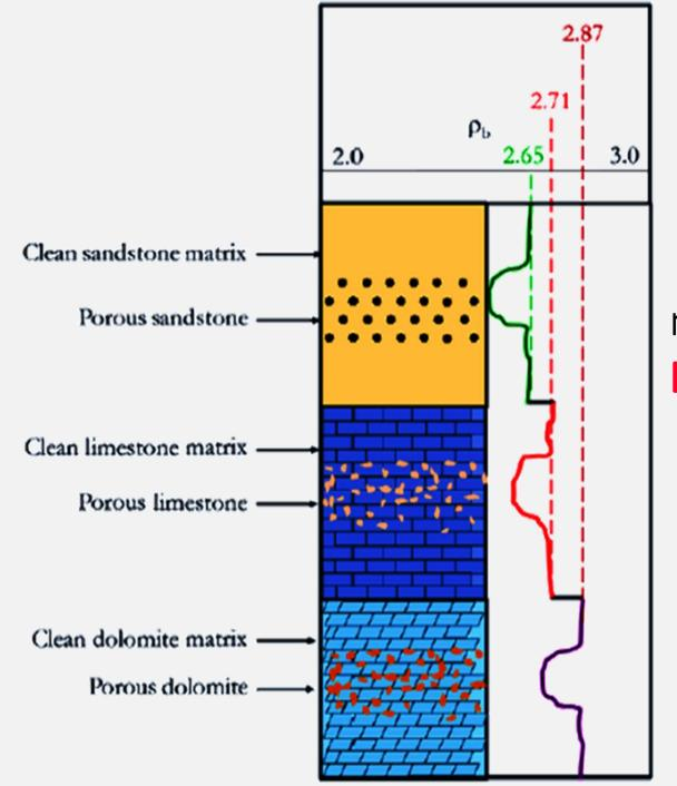
The bulk density decreases due to the effect of the pore spaces (porosity) in each lithology
