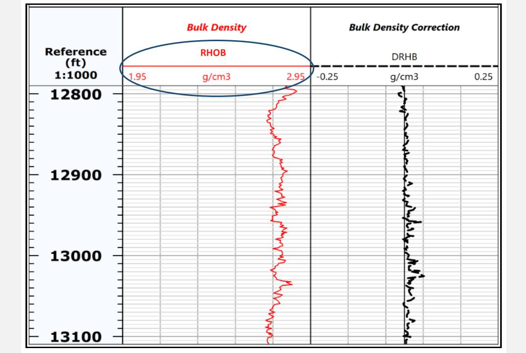
The unit for pb is g/cc and density porosity is in porosity units (pu). When a sandstone matrix density is used for calculating density porosity, it is called the sandstone porosity unit (SSPU or **SPU)**; when a limestone matrix density is used for density porosity calculations, the porosity unit is the limestone porosity unit (LPU).
