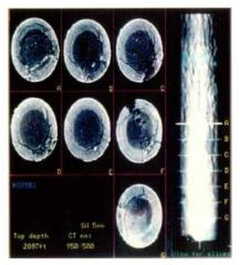
is one of the most widely used imaging techniques, which permits visualization of internal rock features. It was first introduced as a radiological imaging technique by Hounsfield in 1972.
