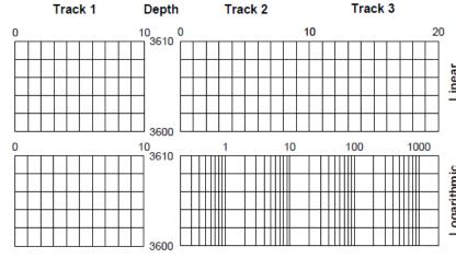
tracks. This allows the display of readings from 0.2 to 2000 ohm.m.
