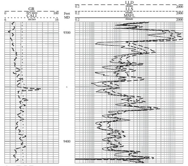
The following ratios are needed for work on the tornado chart (Figure 6), and the values represented are picked from the log as shown above:
