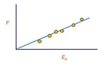
The above interpretation technique is useful in that, if a simple linear relationship for equation above is expected for a reservoir and show later the actual plot turns out to be non-linear, then this deviation can itself be diagnostic in determining the actual drive mechanisms in the reservoir. For instance, equation above may turn out to be nonlinear because there is an unsuspected water influx into the reservoir, helping to maintain the pressure.
