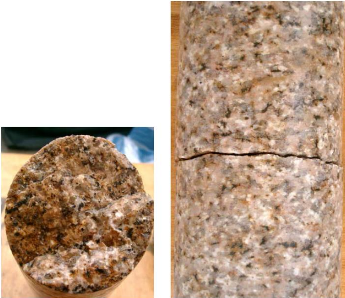
Figure 4. Drilling induced fractures
