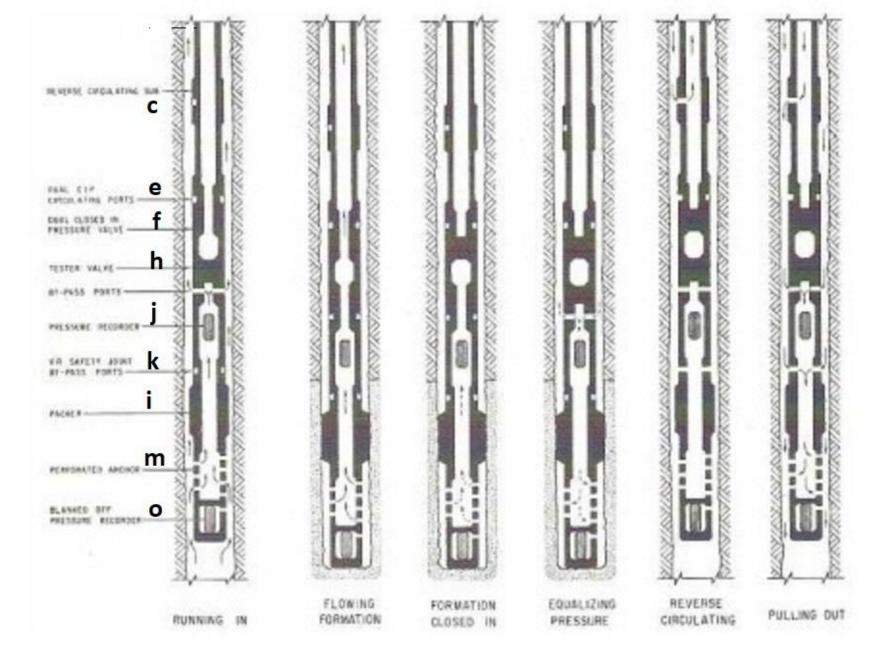
Figure -25: Fluid passage diagram, open-hole drill stem test.
