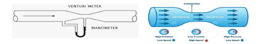
The Venturi effects is the reduction in fluid pressure that results when a fluid flows through a constricted section (or choke) of a pipe
