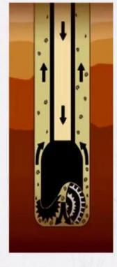
The drill string is turned at surface, which turns the bit at the bottom of the hole.
