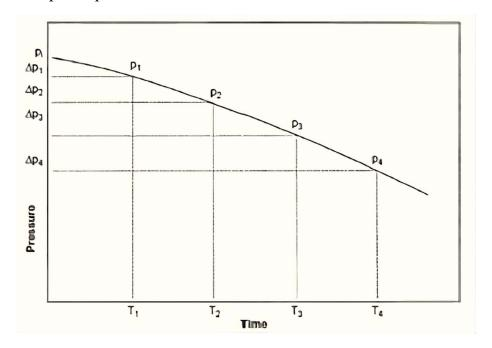
In calculating the cumulative water influx into a reservoir at successive intervals, it is necessary to calculate the total water influx from the beginning.
