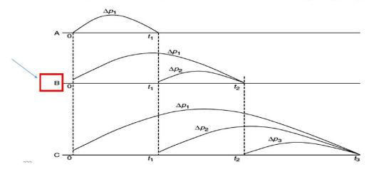
Step 3. A third pressure drop of  $\Delta p_3 = p_2 - p_3$  would cause an additional water influx as illustrated in section C . The cumulative (total) water influx can then be calculated from:
