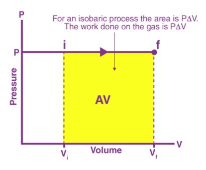
**Ex (3):** 0.2 kg of fluid initially at a temperature of 165 °C, expands reversibly at a constant pressure of 7 bar until the volume is doubled. Find the final temperature, work done and heat transfer.
