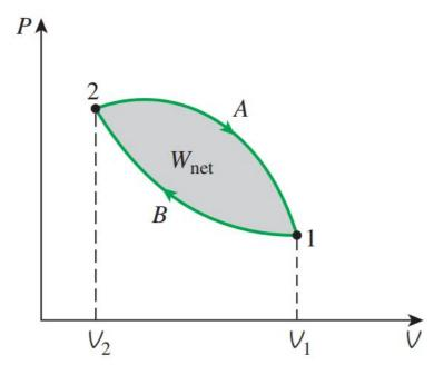
The net work done during a cycle is the difference between the work done by the system and the work done on the system.
