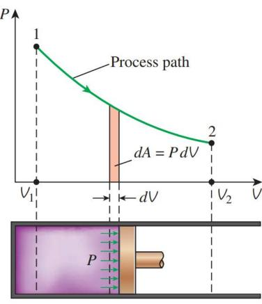
The area under the process curve on a P-V diagram represents the boundary work.
