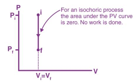
Ex (2): A fluid in a closed vessel of a fixed volume of 0.14 m3, at pressure of 10 bar and temperature of 250 °C. If the vessel is cooled so that the pressure falls to 3.5 bar, determine the final temperature and the heat transferred R=0.278 kJ/kg K, Cv=0.718 kJ/kg K
