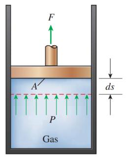
A gas does a differential amount of work  $\delta W_b$  as it forces the piston to move by a differential amount ds.
