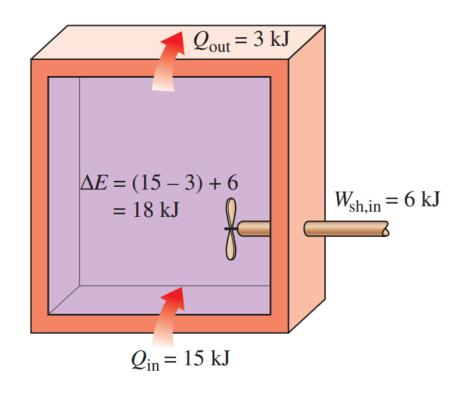
The work (boundary) done on an adiabatic system is equal to the increase in the energy of the system. The work (boundary) done on an adiabatic system is equal to the increase in the energy of the system. The energy change of a system during a process is equal to the net work and heat transfer between the system and its surroundings.
