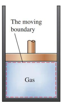
The work associated with a moving boundary is called boundary work.
