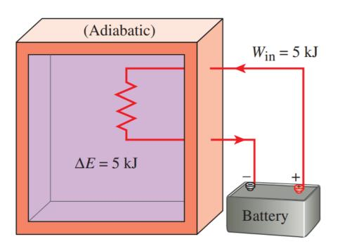
The work (electrical) done on an adiabatic system is equal to the increase in the energy of the system.
