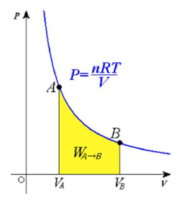
**Ex (4):** A quantity of O2 gas at a pressure of 5 bar, volume of 0.1 m3 and temperature of 1227 oC expands isothermally until its pressure reduces to 1 bar. It is then cooled isobarically to the original volume. Find the change in internal energy, work done and heat rejected during each process.
