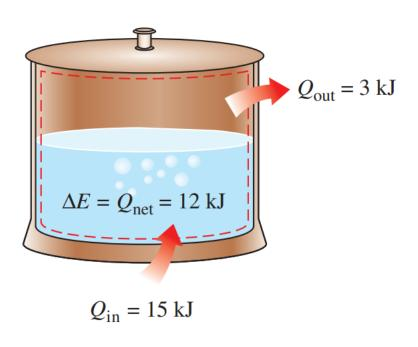
In the absence of any work interactions, the energy change of a system is equal to the net heat transfer.
