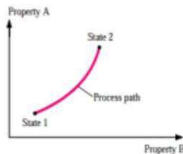
Fig. 1.7 A process between states 1 and 2 and a process path
