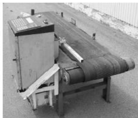
Fig. 6.1.1. A flat belt conveyor with drive control
