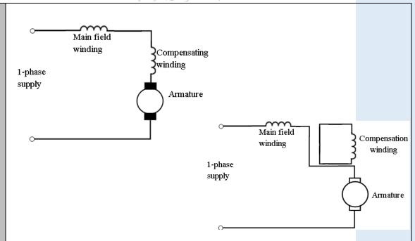
Like DC series motor. The speed of a universal motor is low at full load and very high at no load. Usually, gears trains are used to get the required speed on required load
