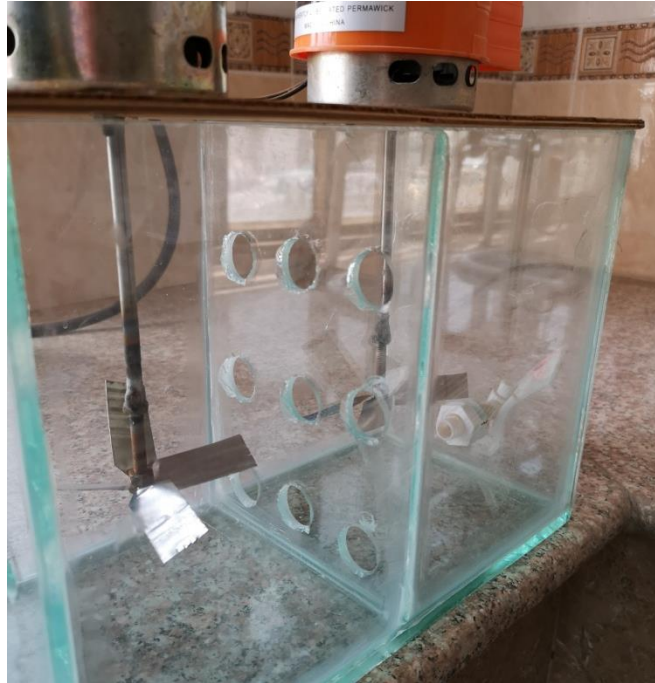
Figure 3 The distribution of the holes in the baffles separated the flocculation stages.
