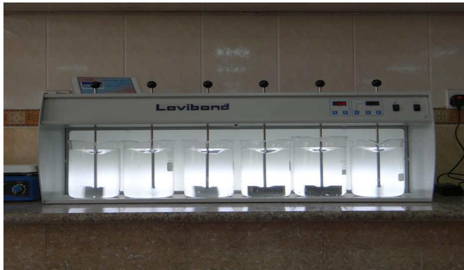
Figure 2 A photograph showing jar test apparatus used in the research
