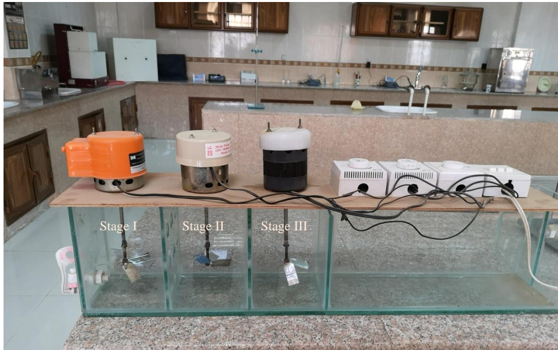
Figure 1 A photograph showing the multistage flocculation model
