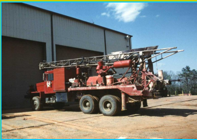
Wire line Rig for Kaolin Mines, Macon, GA
