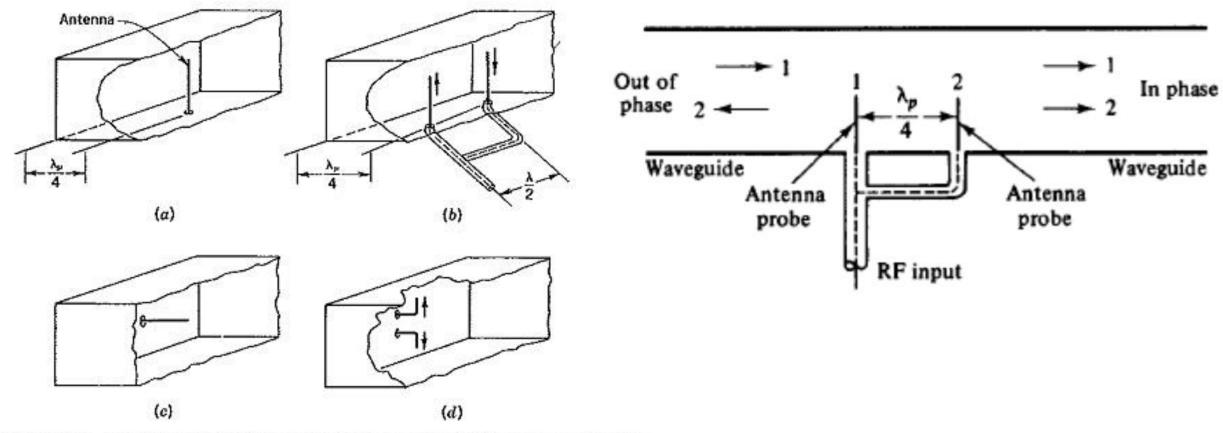
FIGURE 10-15 Methods of exciting common modes in rectangular waveguides.
