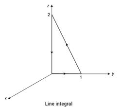
Along the path BC, dx = 0, x = 0; y varies from 1 to 0 and z varies from 0 to 2.
