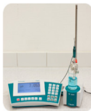
Figure 14.13.1: A pH meter is a laboratory device that provides quick, accurate measurements of the pH of solutions. (CC BY-NC; CK-12)
