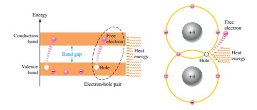
A pure Silicon crystal at room temperature takes heat from surrounding air, causing some valence electrons to gain sufficient energy to jump the gap from the valence band into the conduction band, becoming free electrons.
