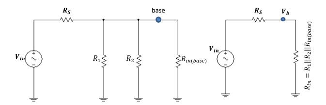
$$V_b = \left(\frac{R_{in}}{R_S + R_{in}}\right) V_{in}$$
