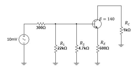
$$r'_{e} = \frac{25mV}{I_{E}} = \frac{25mV}{2.4mA} = 10.4\Omega$$
