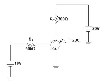
Q-point is defined by  $\,I_{\it C}$  and  $\,V_{\it CE}$
