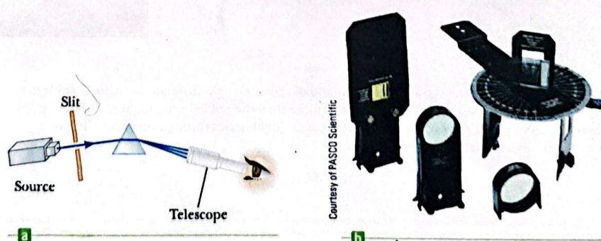
Figure 22.16 (a) A diagram of a prism spectrometer. The colors in the spectrum are viewed through a telescope. (b) A prism spectrometer with interchangeable components.
