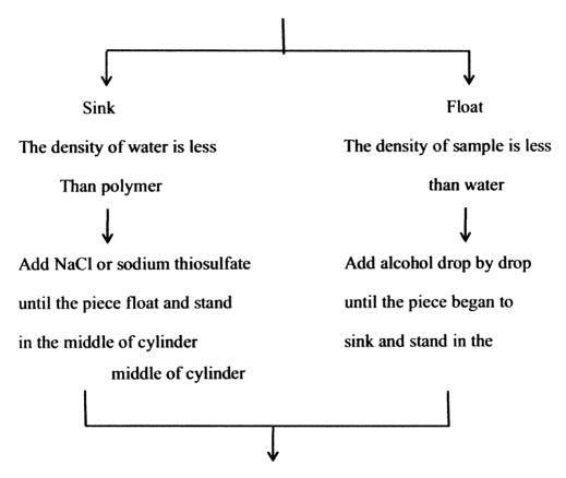
Measure the density of the solution by standard method density of solution = density of polymer check your result with table (4)
