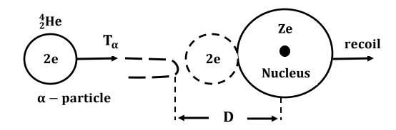
When an  $\alpha$  – particle is far from given nucleus it has only kinetic energy  $(T_{\alpha})$ . It comes closest to the nucleus in a head – on collision.
