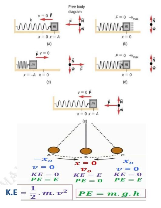
When a body oscillates at a distance X from its equilibrium position, where F represents the resultant force acting on the body and equals the restoring force -Kx, according to Hooke's law, expressed as F= -kx. This is derived from Newton's second law.
