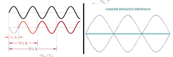
It is evident from the figure that the resultant of the capacitance equals the difference between the capacities of the two overlapping compatible movements, and the peak of one of them is above the bottom of the other. The movements oppose each other, and in this case, they destruct each other and are called destructive interference. In the case of  $a_1=a_2$ , the resultant is zero, as shown in the above figure.
