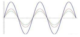
From the above graph, it can be seen that the amplitude of the resulting vibrating motion is equal to the sum of the amplitudes of the two overlapping motions having the same frequency and phase. This means that the two harmonic
