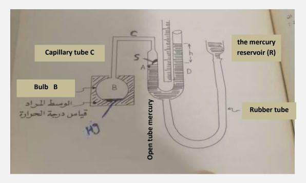
Calibration the thermometer: To calibrate the thermometer with the Celsius scale, the bulb B is placed in crushed ice until the trapped gas becomes thermally balanced with the ice at  $0^{\circ}$  and then the reservoir position is
