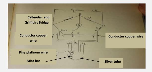
To calibrate this thermometer, the tube containing the platinum wire is placed at known standard temperatures, then its resistance is measured at these degrees. Then the thermometer is placed in the medium with the unknown temperature and its resistance is determined in the same previous way, and from that the unknown temperature can be calculated. If it is:
