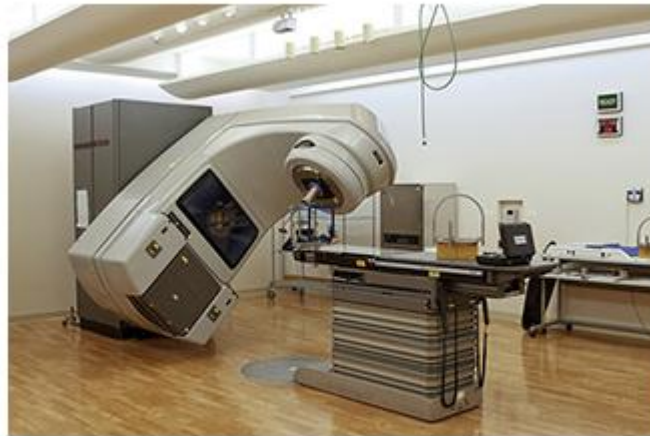
Figure 2. Linear Accelerator. Source: Daniel Sone (Photographer), National Cancer Institute.
