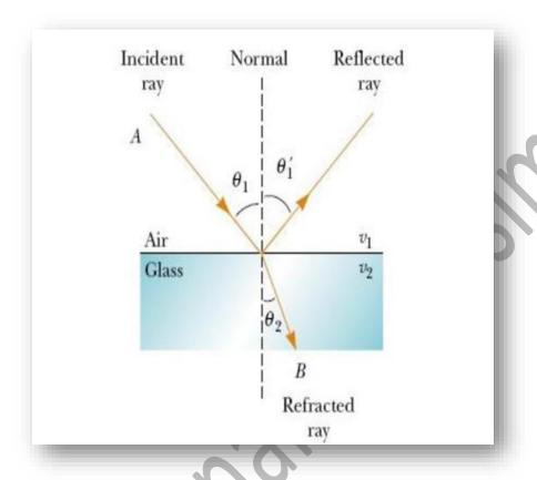
Fig (6): Illustration of the Refracted ray
