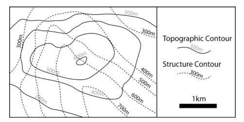
4. (10 MINUTES) The maps below (a and b) shows the outcrop of a coal superposed on topographic contours. Construct structure contours and calculate the strike and dip of the coal in each map. In both cases, assume that the coal is planar.
