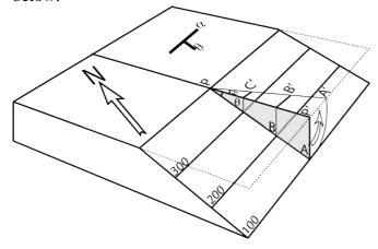
In this case we imagine a vertical cross section that passes through the measurement point (P) of a strike and dip. The section line is oriented perpendicular to strike (so that it shows true dip). This is the plane P-P'-A on the 3D diagram above. The dip is  $\theta$ . In the graphical construction we imagine rotating the cross section 90° around line P-P' so that it lies in the horizontal (map) plane: A rotates onto A', B onto B' etc.
