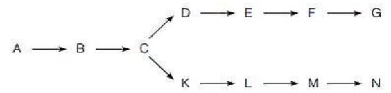
To control the pathways so that G and N keep in balance, high concentrations of G might inhibit the  $C \longrightarrow D$  enzyme or activate  $C \longrightarrow K$  enzyme. Conversely, high concentrations of N might inhibit  $C \longrightarrow K$  enzyme or activate the  $C \longrightarrow D$  enzyme.
