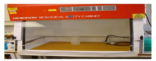
**Class II** - air is filtered and most of it is recirculated through the cabinet. This cabinet protects the work as well as the worker. About 70% of the air is recirculated through filters so that the working area is bathed in clean (almost sterile) air.
