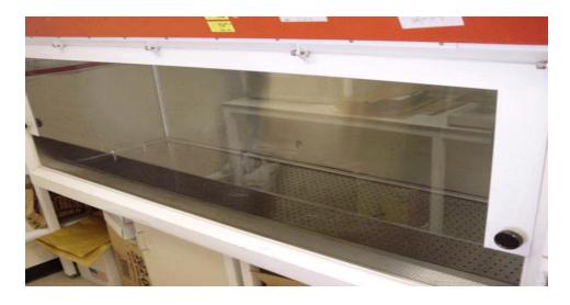
Class III - cabinets are totally enclosed and leak-proof. The operator works with gloves which are sealed into the front of the cabinet by removable gaskets.
