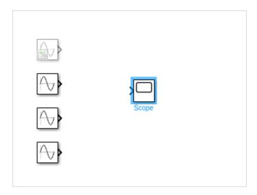
The sine wave has one output and the scope block has one input. We have four sine waves displayed. We have to change the parameters of scope block to take four inputs.
