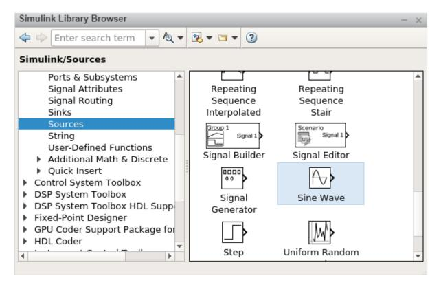
To move the sine wave to your model, select the block and drag it inside your model workspace. We want to display the sine wave and here, we have taken four sign wave in our model workspace as shown below:
