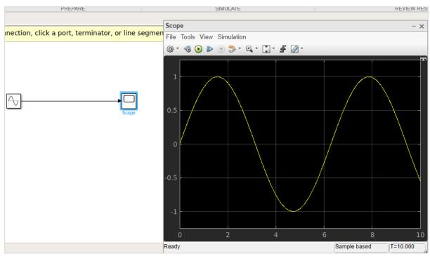
Let us now add delay for the sine wave. We will make use of transport delay block from continuous library as shown below:
