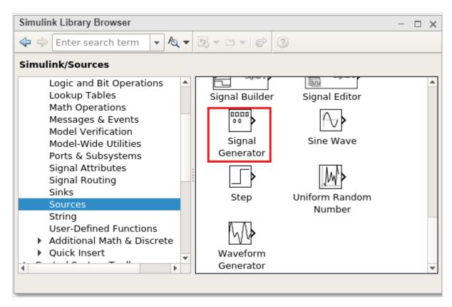
Select the Signal Generator and drag it to get inside the blank model as shown below:
