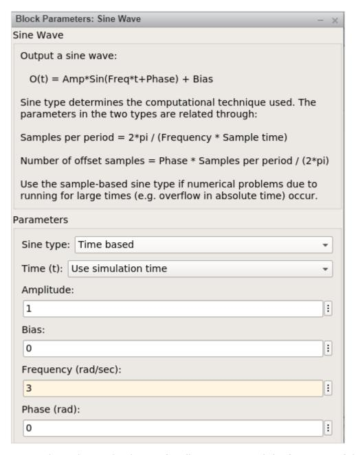
We are going to keep the amplitude as 1 for all sine waves and the frequency of the first sine wave is 1, second one is 3, third one is 6 and the last one is 10.
