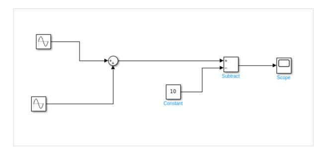
Click on the run button to compile. Right Click on scope block to see the signal plotted.
