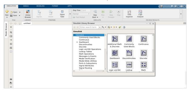
Let us select the block that we want to build a OR gate. We need two constant blocks to act as inputs, a logic operator block and a display block.
