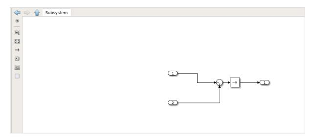
Click on the upward arrow close to the subsystem to get back to the model.
