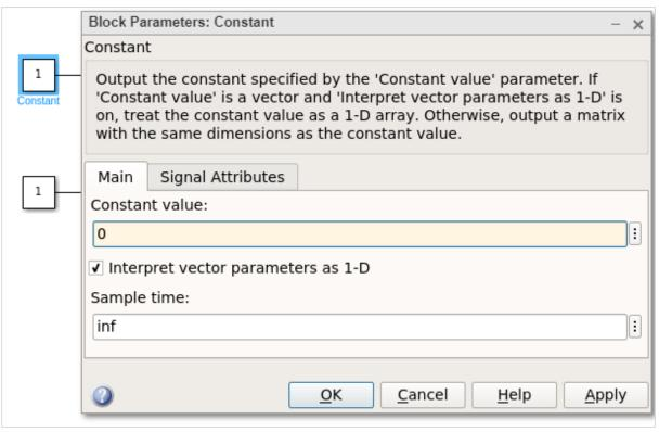
After changing the values of constant to 0, the output will become 0 when you run the model. The output is as shown below:
