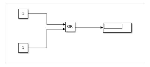
For an OR gate if the inputs are 1,1 the output will be 1. If the inputs are 0,0 the output will be 0. Right now, the constant has values 1,1. Let us run the model to see the output as shown below:
