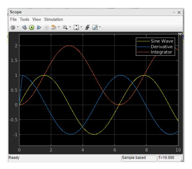
So, we have three signals sine wave, derivative and integrator.
