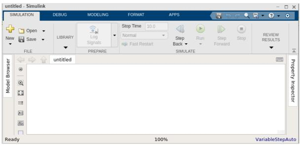
We need a constant block, a MATLAB function block and a display block for the output.
