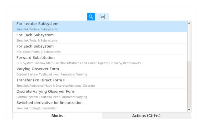
Select the for Iterator subsystem block and add to your model. Next, we need display block as shown below:
