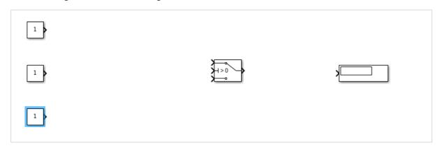
Let us now connect the lines with each block. So you can see that the constant block has one output and the switch has three inputs and one output. We are going to connect them to the display block.
