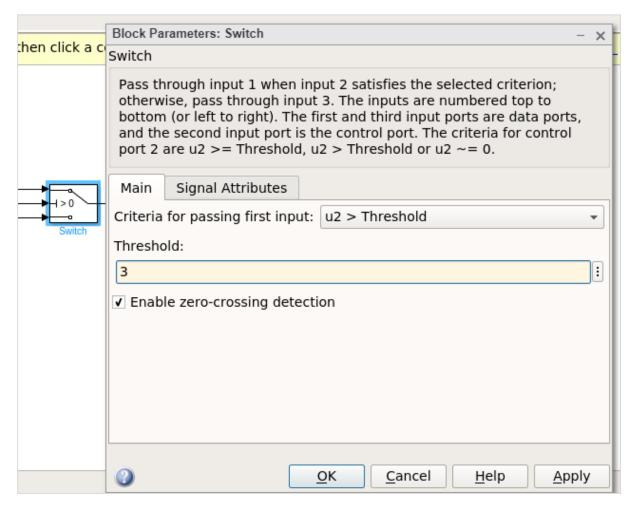
The threshold value given is 3. Click on OK to update the threshold. Now the threshold value is seen inside the switch block as shown below:
