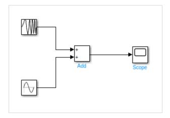
Double click chirp signal and change the initial frequency from 0.1 to 0.05 and click on Ok button.
