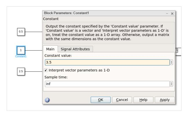
The value is changed from 1 to 3.5. Click on OK and run the model to see the output in the display:
